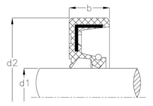
$\begin{array}{ll} b & = 7 \\ d1 & = 17 \\ d2 & = 32 \\ Material = NBR \end{array}$
